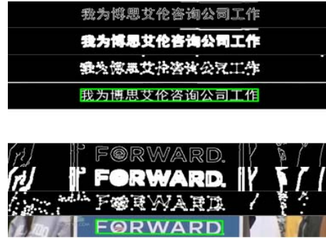
Fig. 5 Two samples of using canny rate criterion. Four images are respectively canny map, dilated canny map, the graph which stores the structure of characters and the final text line detected.
