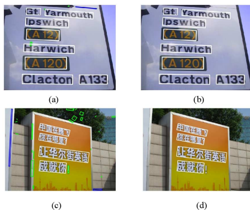
Fig. 12. False positive removal. (a), (c) False positives marked by green color and blue color. (b), (d) The effect of rule-1 and rule-2 where both the false positives are eliminated..
